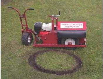
Allows for tight turns and curves and the ability to cut small diameter tree rings down to 18" diameter.
