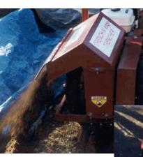
Dual side discharge, sends soil into or out of flower bed, from either direction
